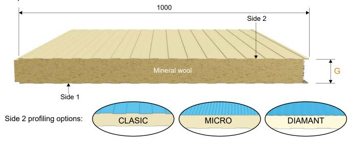
Depending on the thickness of the insulation, the panel fire resistance may vary.
